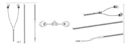
The figures depict a preferred zipper earphone cable assembly comprising first and second cables that include means for releasable attachment with one another. Each cable can be operably coupled to an earphone at a first end and a headphone jack suitable for connection to an audio playing device at the other end. The head phone jack can be any suitable jack including a 6.35 mm jack, 3.5 mm miniature jack, or a 2.5 mm subminiature jack, for example.
